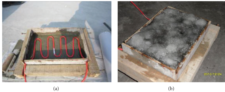
FIGURE 11: Laying of heating cable in the laboratory experiment.
